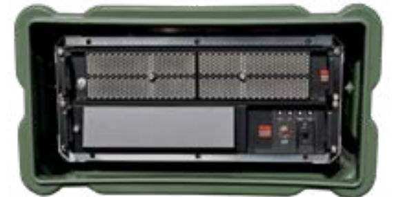
The P2896R installed into a case with Westek's M2316R 2U UPS
